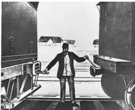
Link-and-pin system AmericanHeritage.com
